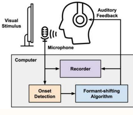
**Pitch/Formant-shifting** algorithm Audapter (Cai et al., 2008; Tourville et al., 2013)
