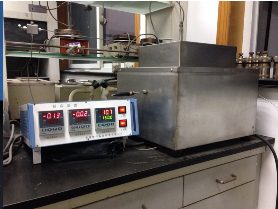
High Pressure Reactor
